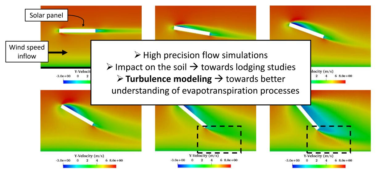
(Micro-climate simulation in case of an obstacle, 13-hours simulation « summer » conditions)
